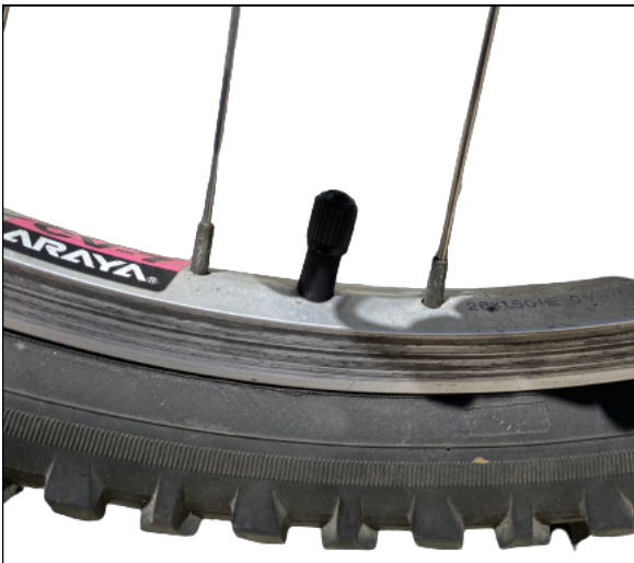
Example of a Schrader valve.
